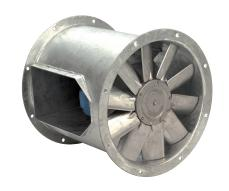
A range of bifurcated axial fans, specially developed with motor out of the airstream to handle more hostile air movement applications.
